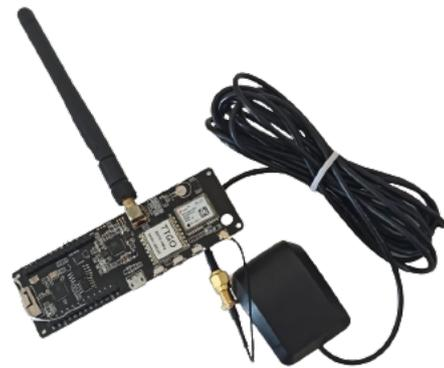
Figura 2 – Lillygo Tbeam V1.1 com antena LoRa e GPS
